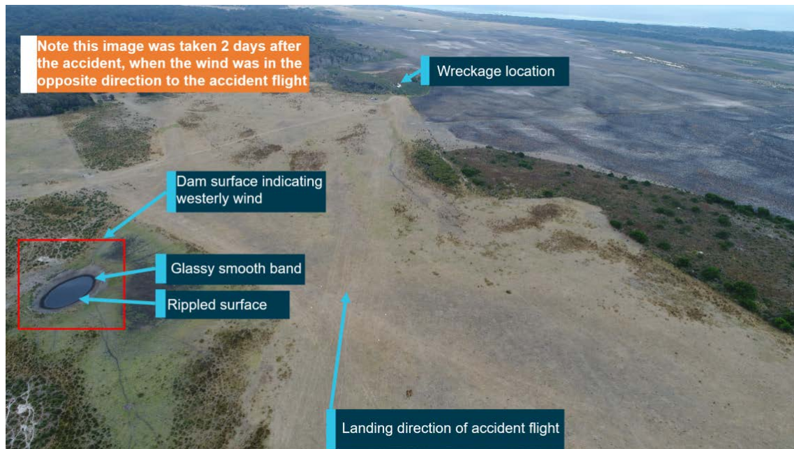
Figure 3: Airfield looking in the landing direction (west) from runway threshold, showing dam surface. Note: image was taken 2 days after the accident, in a westerly wind
